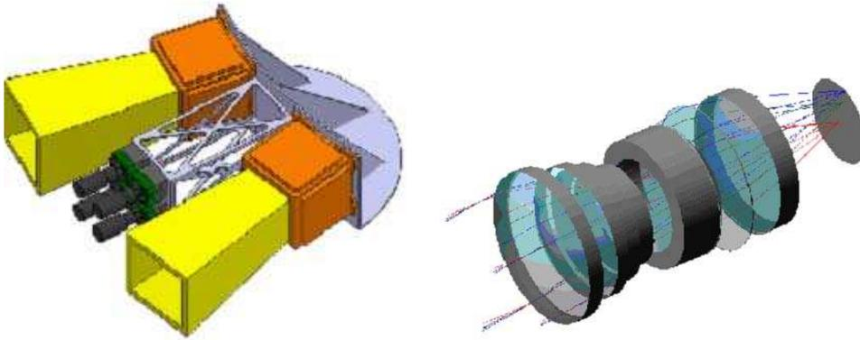
Figure 3: Photometers and video cameras layout (left) and optical design (right).
