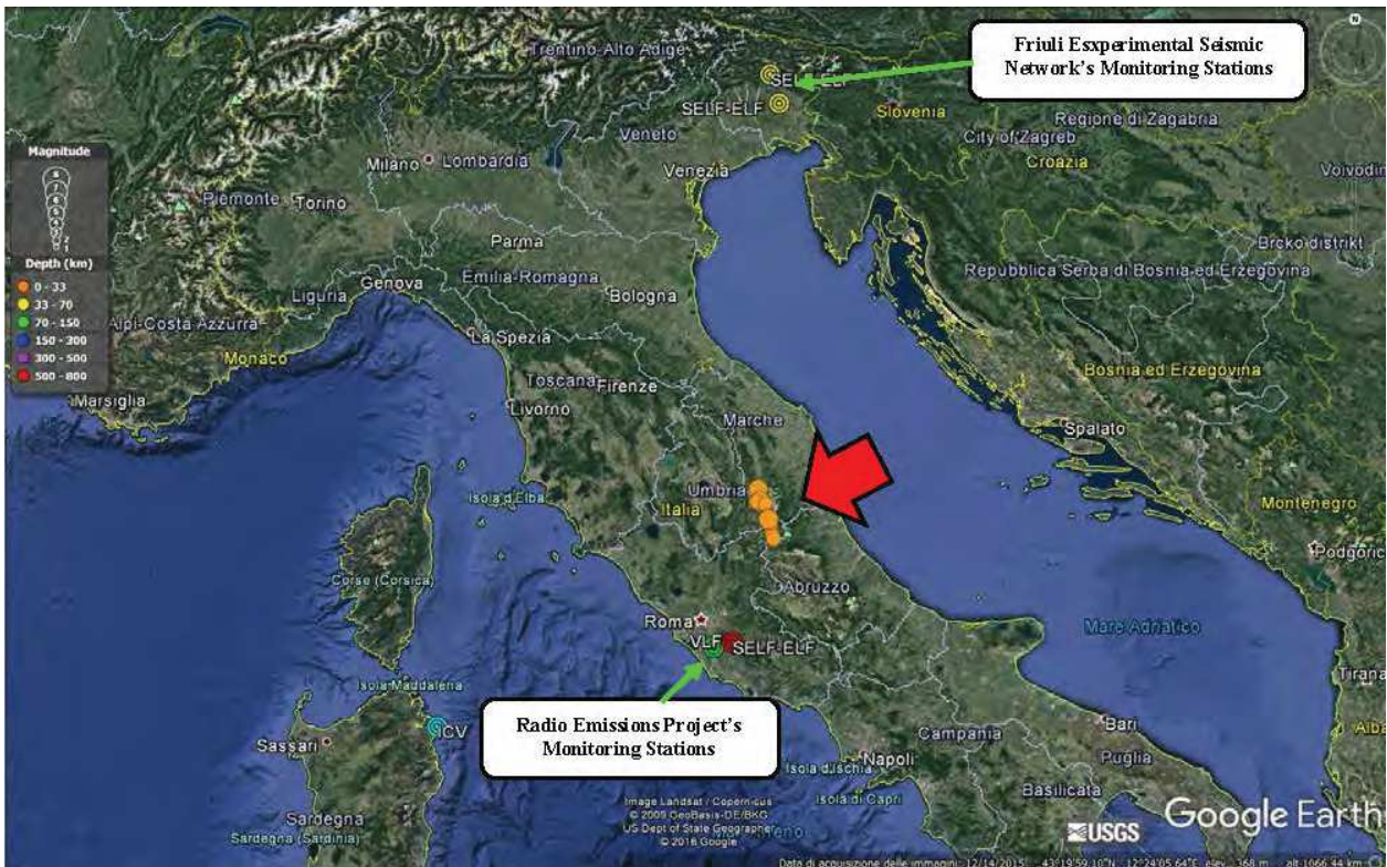
Fig. 1 – Central Italy earthquakes: The picture shows (red arrow) the seismic epicentres (orange circles) of M5+ earthquakes occurred in Central Italy between 24 August 2016 and 18 January 2017. At the top, the two yellow round icons indicate the two SELF-ELF electromagnetic monitoring stations realized by "Friuli Experimental Seismic Network" (FESN) located in Trasaghis, Udine (the top one) and at Pasian Di Prato, Udine (the lower). The two colored icons visible on the bottom of the image indicate the electromagnetic monitoring stations of Radio Emissions Project located at Albano Laziale, Roma (the green icon) and in Lariano, Rome (the red icon).
