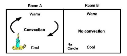
2. Draw the diagram on the board. Ask the students in which room the air will circulate by convection currents. Emphasize that in room A, the difference in temperature caused by the candle will help circulate the air by convection. Ask the students in which directions they air will circulate. Warm air will rise, cool down and move to the left. When the air cools it will then descend.
