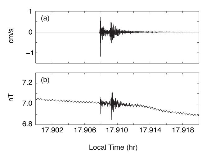
**Fig. 6.** Data during a nearby earthquake is plotted from station HDW, Honeydew. (a) normalized geophone data. (b) normalized data from the vertical induction coil. The low-amplitude periodic signal in (b) is a nearby cultural noise source that appears during the day. Time is given in local time as the number of hours since midnight, 25 March 2006. System response to the P and S waves are clearly seen in both plots. See Karakelian et al. (2002) for additional coseismic signals.
