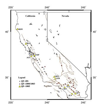
**Fig. 1.** A map of sensor locations in CalMagNet. The QF-1005 reference stations are shown as yellow triangles and labeled with station codes. Light blue and red triangles represent QF-HS and QF-1000/1003 stations respectively. Station locations coarsely reflect the San Andreas and adjacent fault systems, and are placed in high probability earthquake regions.
