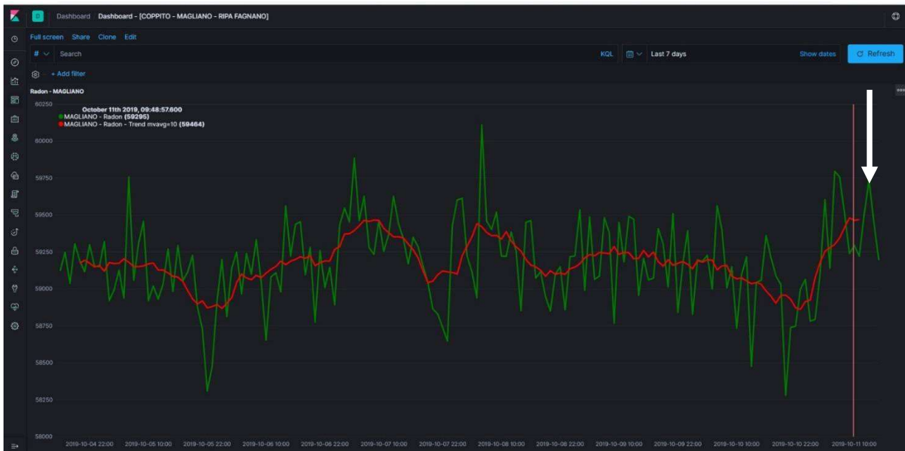
Fig. 5 – Gas Concentration Rn_{222} recorded between 4 and October 11, 2019 by the second detector located in pairs range (AQ). At the top it is possible to observe the counting rate relative to the graph of Rn_{222} gas recorded by a second detector located in the range of Coppito monitoring station (AQ). The data confirm the reliability of the anomalies observed on the moving average of the two range sensors located in the east of L'Aquila. Credits: Permanent Foundation G. Giuliani.
