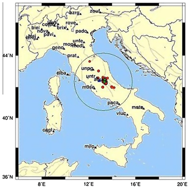
Fig. 2. Map of GPS stations (black triangles) located in Italy. Encircled are stations Unpg , Untr , Aqui , M0se and Paca . Red circles highlight the epicenters of earthquakes (EQs) of magnitude M > 4 occurred in Central Italy for the period 01 January–30 April 2009. Green circle denotes the epicenter of the main EQ shock occurred on 6 April 2009. (For interpretation of the references to color in this figure legend, the reader is referred to the web version of this article.)
