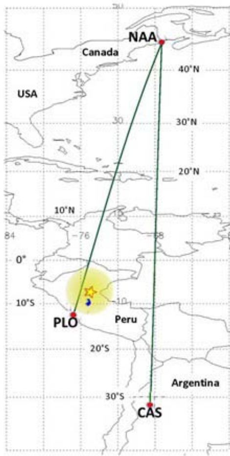
Figure 2. Great-Circle projection of the VLF radiowave propagation paths used in the analysis from the transmitter station NAA in Northern Canada to receiver stations PLO and CAS in Peru and Argentina, respectively.
