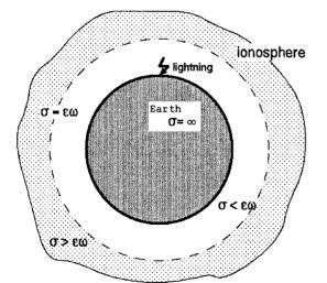
Fig. 1. Configuration of the Earth-ionosphere cavity.
