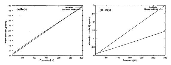
Fig. 5. Comparison of propagation constant. (a) refers to the propagation constant (real part), while (b) the imaginary part, indicating attenuation constant. Two models are compared; our model and Nickolaenko and Hayakawa [11]
