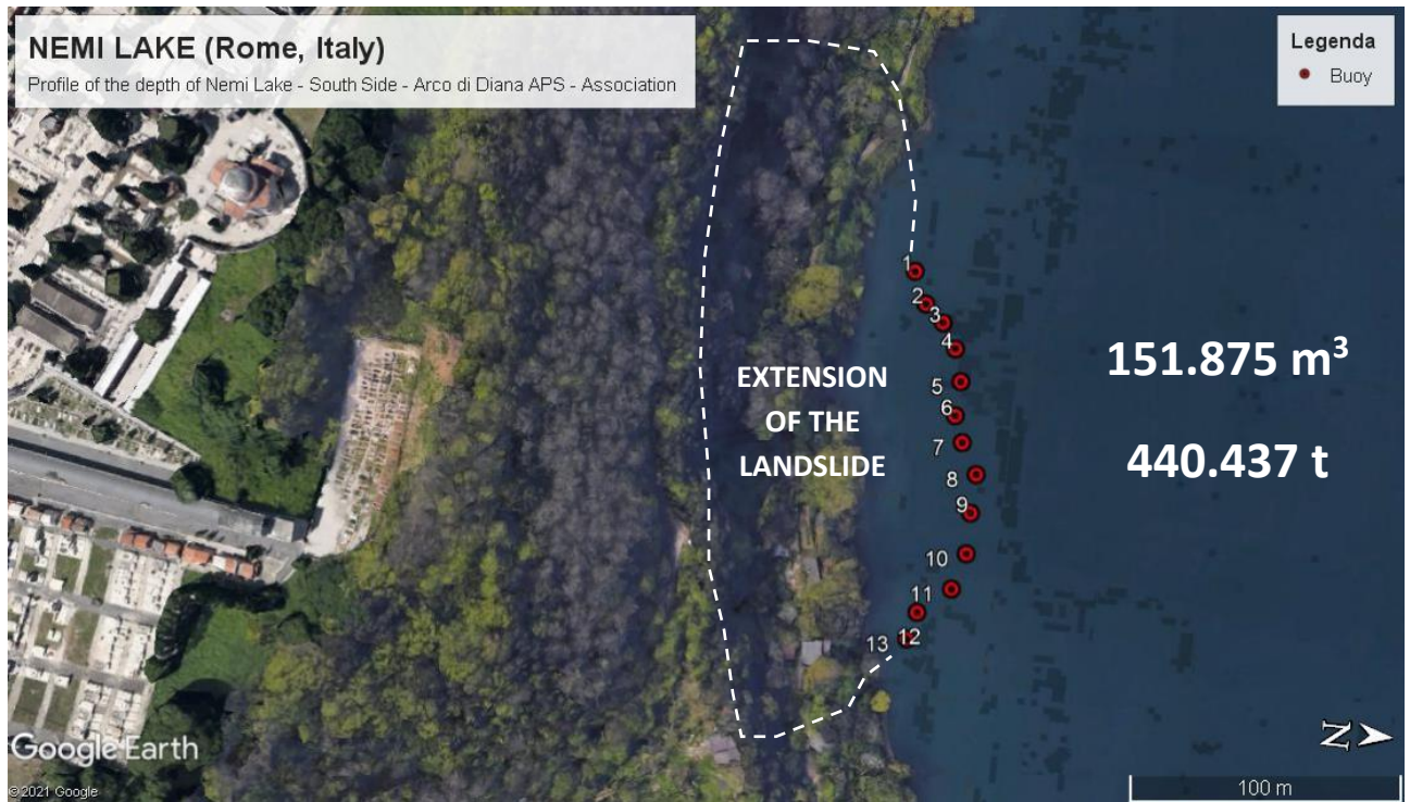
Fig. 10 - Extent of the landslide highlighted both in the water and on the shore. It measures 225 meters long and 100 meters wide (compared to the rock face). Credits: Arco di Diana APS - Google Earth Pro.
