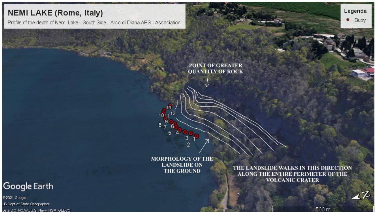
Fig. 15 - Satellite and three-dimensional map of the landslide area (volcanic crater of Nemi Lake). We observe the trend of the rocks present on the ground, located outside the lake mirror. It is evident that in this point there was a greater amount of rock then collapsed towards the ground, such as to move the entire surface of the soil and with it also what had once been built by man. Credits: Arco di Diana APS - Google Earth Pro.
