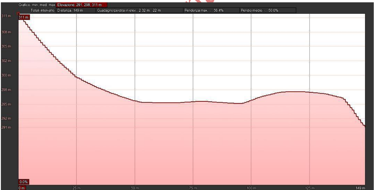
Scheme A – Terrain elevation profile of the geographical area downstream from the access to the cistern. Note how the access is located at about 311 meters above sea level and that the level of the adjacent lake mirror (Lake Albano) is 291 meters above sea level, at a current height difference of 21 ~ 22 meters with respect to the access point of the cistern at a distance of about 149 meters. Credits: Google Earth Pro, Daniele Cataldi.
